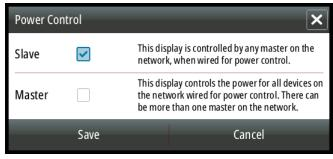
Set to 'Slave' if the yellow wire is connected to ignition or to a stand-alone switch that applies 12V/24V. Set to Master to make this device turn on other devices when powered up.
