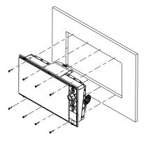
Check the fit of the display, and file away remaining obstructions. Secure the display with the supplied screws. Once screws are fully tightened, ensure there is complete contact with the mounting surface. If machine screws are required, use only M2.5 (3/32") size with a head diameter no greater than 5.6mm (7/32").
