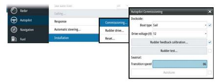
When the autopilot computer is delivered from factory AND ANY TIME AFTER AN AUTOPILOT RESET HAS BEEN PERFORMED, you will have to run a complete setup again.
