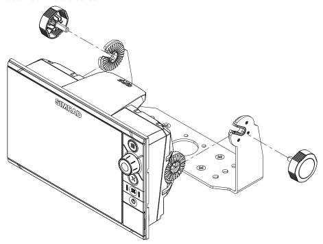
Mount the display to the bracket using the knobs. Hand tighten only. The ratchet teeth in the bracket and display case ensure a positive grip and prevent the unit changing from the desired angle.
