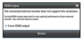
Alternatively, 'Force HDMI output' may be selected in Settings/Advanced/Features. The unit will need to restart to apply the change.
