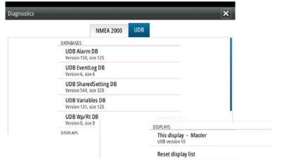
The 'Reset Display List' can be used to refresh the list of connected displays and their UDB version.
