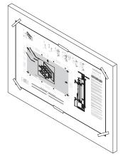
Check the template for scaling accuracy, using a tape measure or ruler against the ruler printed on the template.
