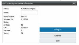
All devices allow allocation of an instance number via the **Configure** option. Set unique instance numbers on any identical devices on the network. The **Data** option shows all data being output by the device. Some devices will show additional option(s) specific to the device - the RC42 illustrated above has a **Calibration** option, to allow easy setup of this device which does not have it's own user interface.
