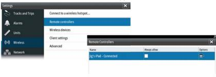
Selecting 'Always allow' will mean the device can automatically connect without needing a password each time. This menu also allows disconnection of devices that no longer require access.
