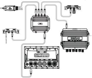
→ **Note:** some ethernet devices are equiped with two or more ethernet ports, which allow connection of additional devices, and may eliminate the need for an extra NEP-2.
