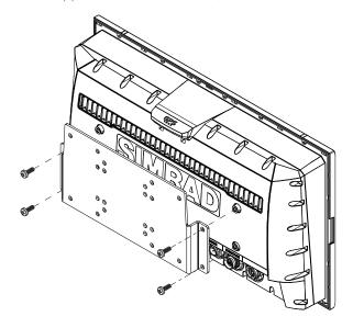
**Warning:** VESA bracket used should be of suitable strength and materials to suit the harsh marine environment. Some standard domestic TV style brackets will not suit potential G-forces applied, and could result in the display coming loose in rough conditions. Use a bracket overrated for the weight and size of the NSS16 evo2.
