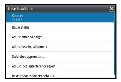
→ **Note:** some radar like the broadband 4G and Halo support dual radar mode, and therefore are represented twice in the source list, with an A and B suffix.
