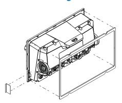
Fit the small self adhesive decal to right side of unit, covering rubber tab of SD card reader gasket. Then attach self adhesive foam gasket to rear of display.
